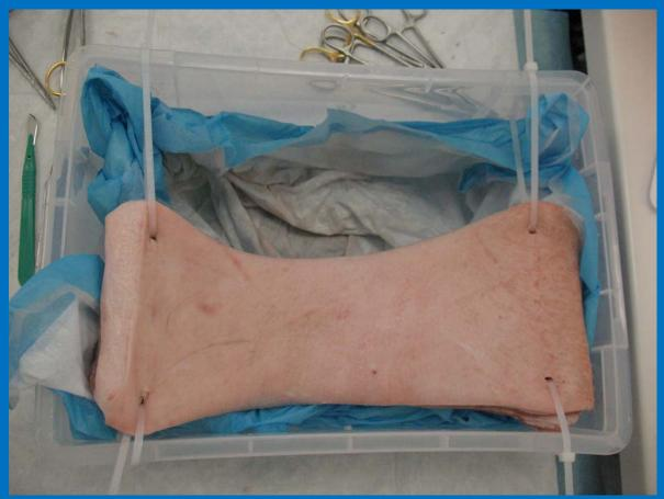
Suspend pork side using cable ties through the drilled holes on the side of the box
