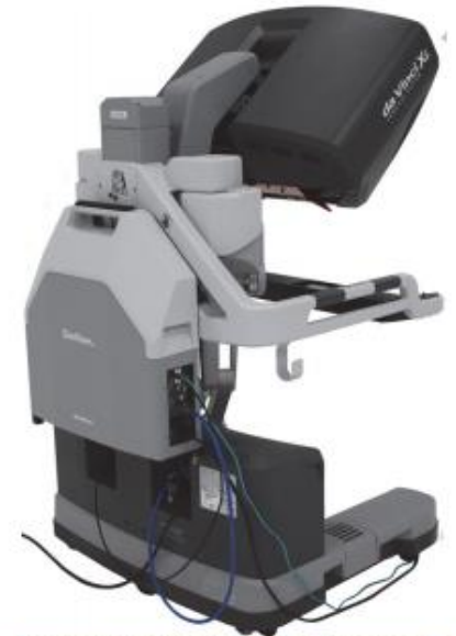
Simulator mounted on back of Surgeon Console
